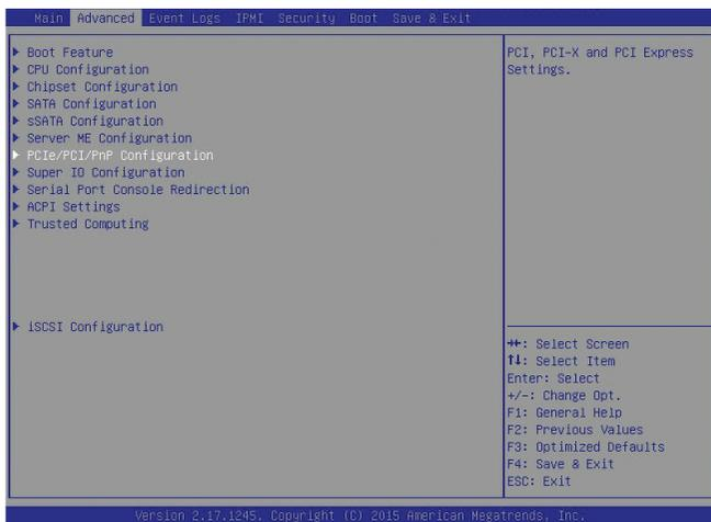
**Warning:** Take Caution when changing the Advanced settings. An incorrect value, a very high DRAM frequency, or an incorrect BIOS timing setting may cause the system to malfunction. When this occurs, restore the setting to the manufacture default setting.
