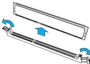
**Warnings:** 1. Please do not use excessive force when pressing the release tabs on the ends of the DIMM socket to avoid causing any damage to the DIMM module or the DIMM socket. 2. Please handle DIMM modules with care. Carefully follow all the instructions given on Page 1 of this chapter to prevent ESD-related damages to your memory modules or components.
