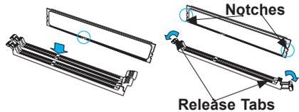
3. Align the key of the DIMM module with the receptive point on the memory slot.
